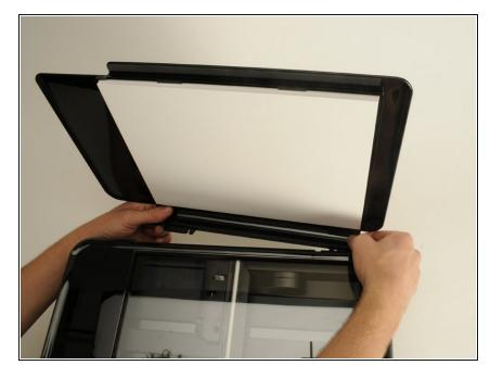
Remove the flap for the scanner. The flap is attached with two clips that can be dislodged by pulling lightly away from the printer.
