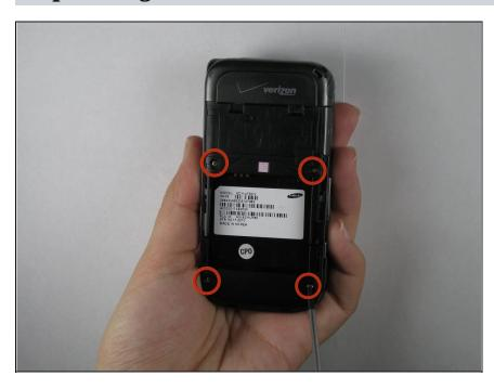
• Remove the (4) 4.2 mm screws from the four corners of the battery slot.
