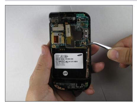
Disconnect connecting cord using tweezers.
