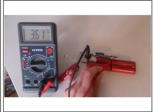
**⚠ Caution:** Lithium-ion batteries can catch fire or explode if they are damaged or short-circuited—especially when they are charged. Be extremely careful not to bend them or short-circuit them with your probes.
