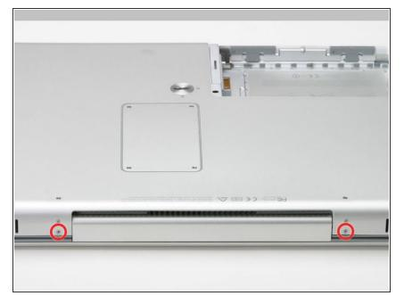
Turn the computer 90 degrees clockwise again, and remove only the bottom screw on either side of the hinge.
