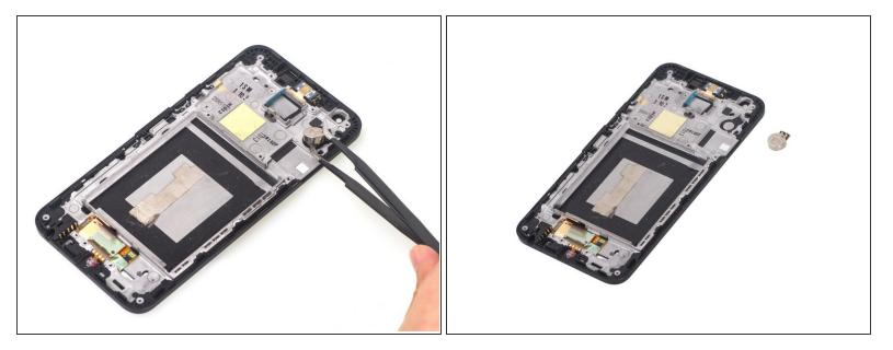
• Adhesive underneath vibration motor is a little bit strong. Pry it up carefully.
