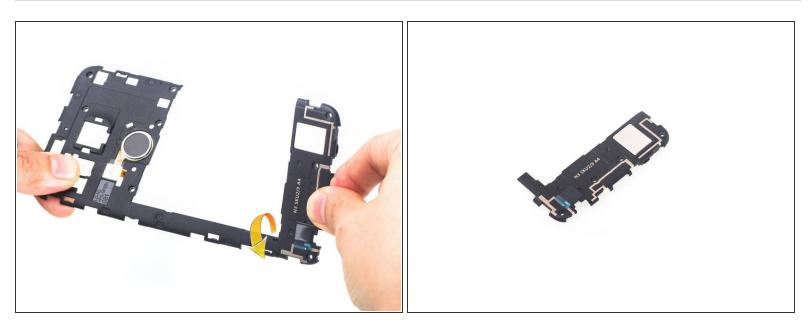
• A flexible clip is here. Loosen it and get the loudspeaker assembly only.
