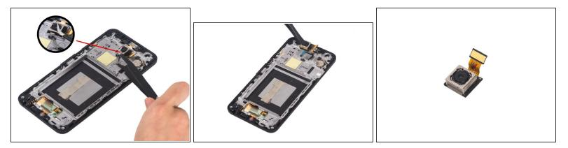
• The adhesive underneath rear camera is strong. Be careful to pry up and remove it.
