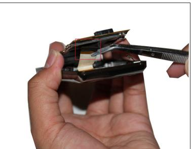
The LCD screen is connected to the bottom of the logic board. Once you lift the logic board use tweezers or a safe prying tool to disconnect the ribbon wire from the LCD screen to the logic board.
