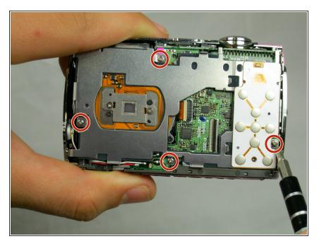
Remove the four 3.8 mm screws located near the bottom right and top left of the LCD base plate.
