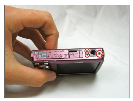
Remove the three 4.1 mm screws on the bottom of the camera.
