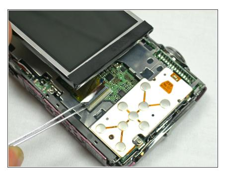
Use the tweezers to lift the ZIF connector which is holding the ribbon cables that connect the LCD screen to the motherboard.
