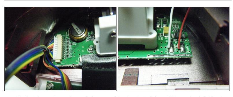
Too bad the speaker and control wires are soldered to the logic board. The speaker is held on by two solder pads. The button control cable connecter may look like it's detachable, but it wouldn't come out. It looks like They get to spend the rest of their lives chained together. But what about the LCD? Is that replaceable?
