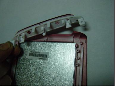
But before the LCD can be removed, the outer snooze button assembly has to come out. It is held on by two screws.
