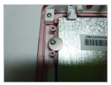
they are 2 metal clamps held on by each one screw, holding the LCD down. Make the screw a little loose and turn each clamp around.
