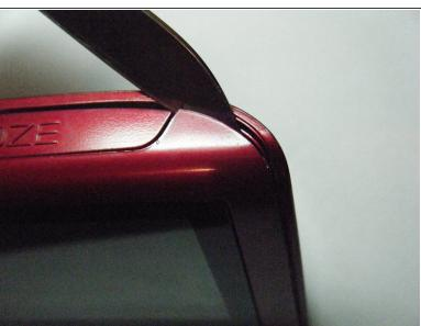
After two outer case screws are removed, The two halves of the case can be easily snapped apart.
