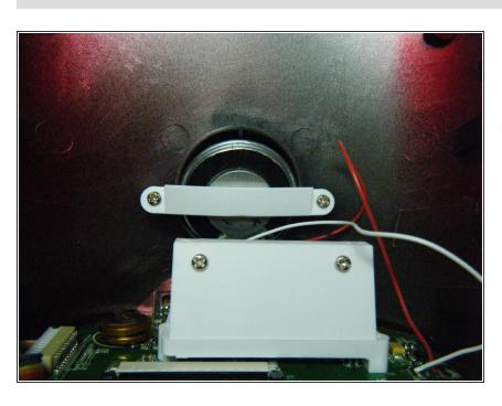
These two plastic pieces hold down the speaker and logic board to the rear case. the screws holding them down must be removed.
