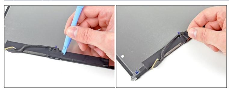
• Remove the small strip of black tape covering the display data cable connector on the LCD.
