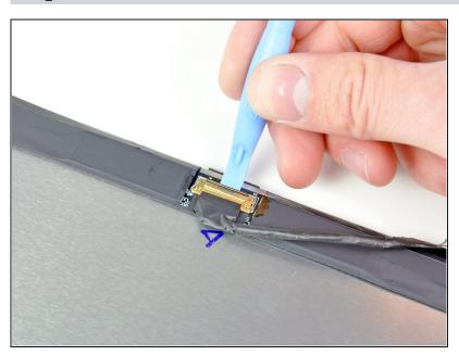
Use the edge of a plastic opening tool to flip up the metal retaining clip on the display data cable connector.
