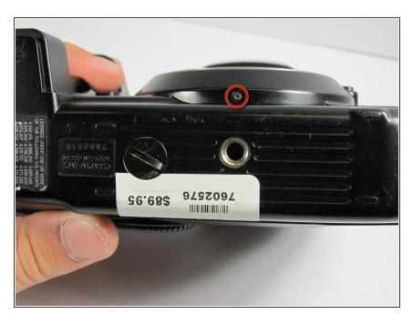
Flip the camera upside down and remove the 5.4mm screw below the lens bezel on the front of the camera.
