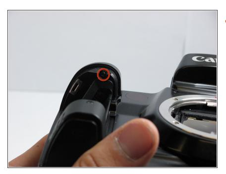
Remove the 6.4mm screw on the top of the inside edge of the battery hole.
