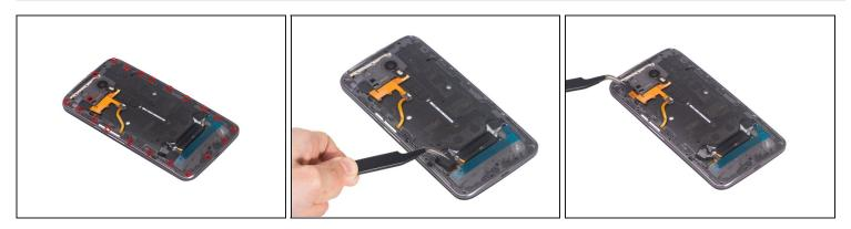
• Use T3 Torx screwdriver to twist off all 21 screws.
