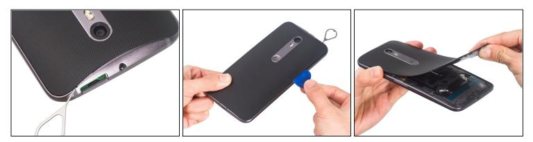
• Insert eject pin to the small hole to open a gap.
