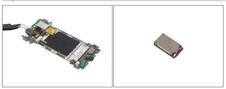
• There is adhesive underneath. Pry up and then remove top speaker.
