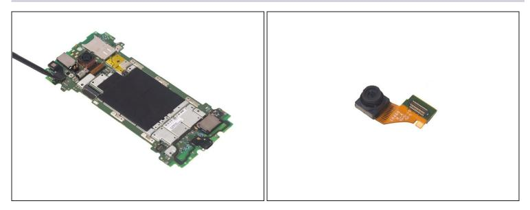
• Release front camera flex and remove it.
