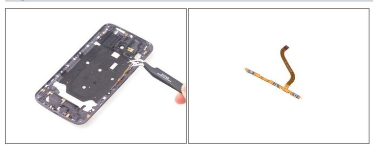
• Pry up and remove power&volume button flex.
