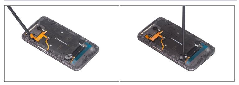
• Release the flashlight flex and battery flex connector.
