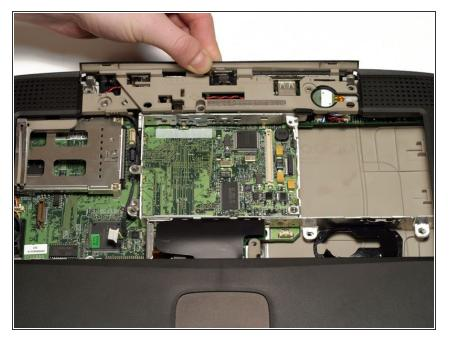
Grasp the upper plastic casing where it locks into the internal frame and pull back. When the plastic tab has cleared the slot that the casing locks into, pull up enough to keep it from locking back into place.
