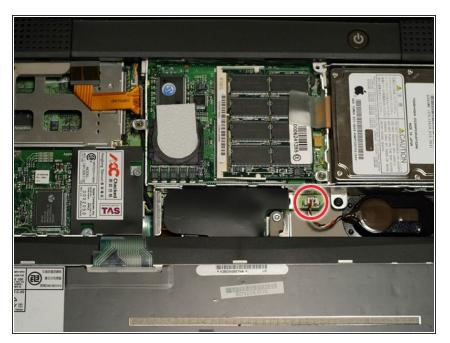
• Pull the battery cable directly up from the logic board.
