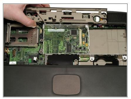
• Remove the upper casing. Note that there are two tabs on the laptop's front that often cause the upper case to stick.
