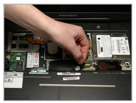
• Remove the battery from its holder by pulling up and to the left.
