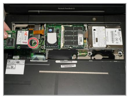
• Disconnect the cable from the right side of the modem.
