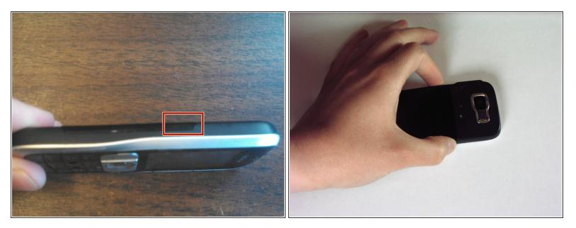
Press each release button on either side of the battery cover and simultaneously remove the battery cover from the phone.
