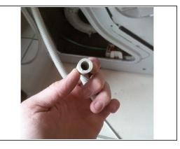
• remove the end of the waterhose( use the flathead screwdriver). and blow the hose out.
