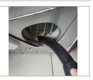
clean out the back of the filterplace. use a wet and drycleaner to do this.
