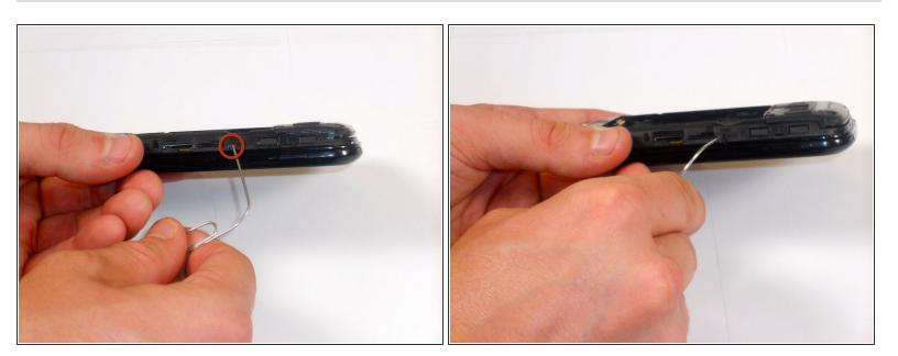
• Using a paperclip or other small pointed tool, press the small red button shown here.
