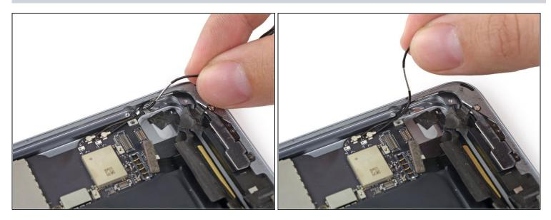
De-route the antenna cable from the retaining clip.
