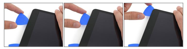
Insert the previous pick deeper into the iPad and slide it away from the camera toward the corner.
