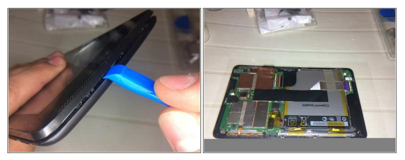
• Make sure your device is turned off. Then with a plastic opening tool, carefully remove the back panel by carefully working your way around the perimeter.
