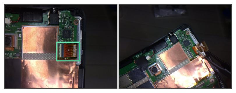
Remove the Display connector from motherboard.
