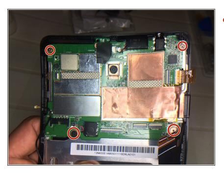
Remove 4screw Philips #0 from motherboard
