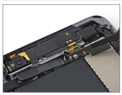
Use a set of <u>tweezers</u> to remove any tape covering the frontfacing camera cable clips.
