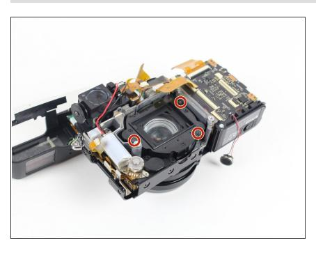
Remove the three 3.5 mm screws on the black lens cover.
