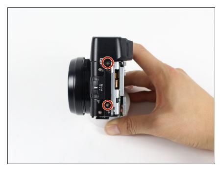
Remove the two 4.5 mm screws on the side of the camera opposite of the battery.
