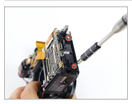
Remove the two 4.0 mm screws located on the side of the camera.
