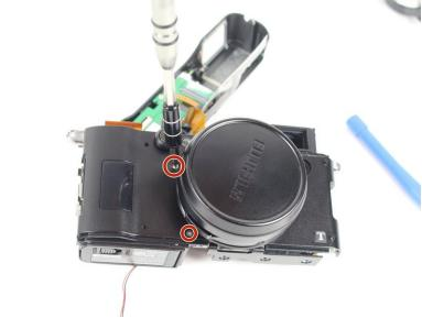
Once the lens has been taken off, flip the camera over and unscrew the two 4.0 mm screws on the front of the camera, next to the lens cover.
