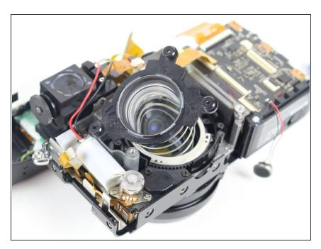
Remove the spring and the lens by gently lifting both the components upwards.
