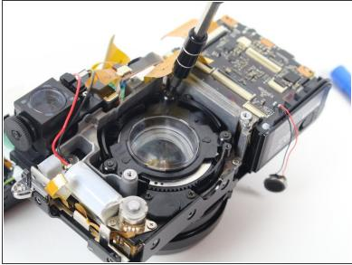
Remove the three 3.5 mm screws on the spring-loaded cover.
