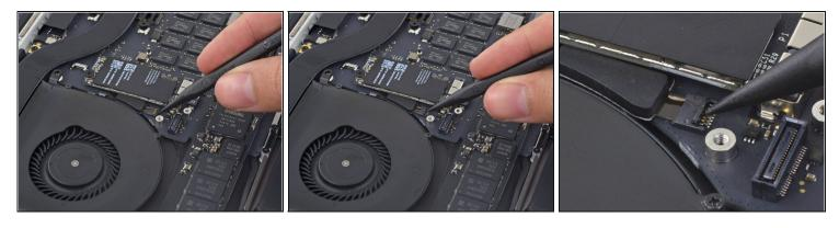
• Use the tip of a spudger to flip up the retaining flap on the right fan ribbon cable ZIF socket.
