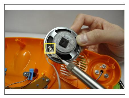
Desolder the electrical connections from the speaker and replace part.
