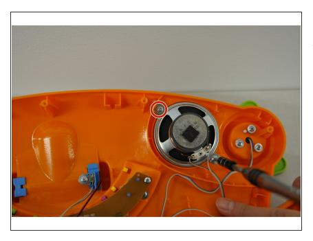
In the top right corner inside the device, unscrew the 2 PH2 screws (5 mm) holding the speaker in place.
