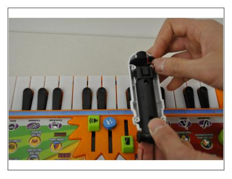
Install new microphone in the device like shown. To reassemble your device, follow these instructions in reverse order.
