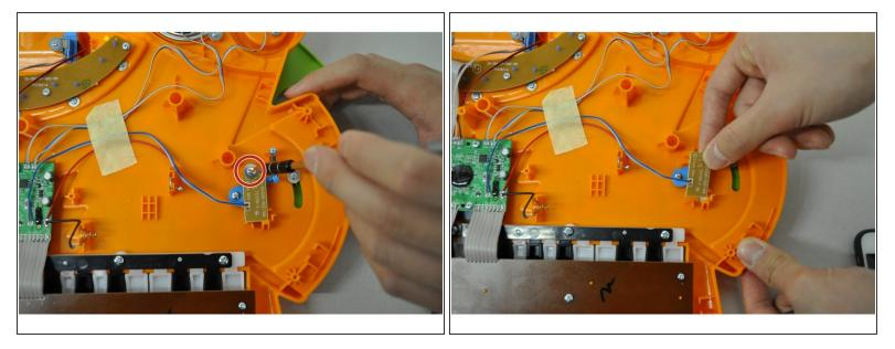
Remove PH2 screw (5 mm) from yellow/gold colored circuit board and pull back to access the whammy component.
