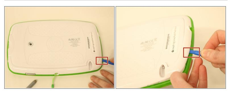
Using a plastic opening tool, pry off the plastic border by inserting it in the space between the green bumper and the white plastic on the edge of the tablet.
