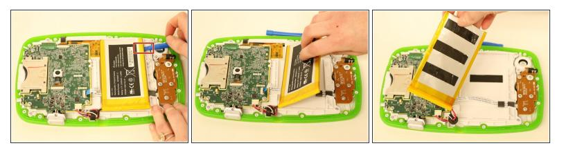
• Wedge a plastic opening tool underneath the battery and lift the battery up.
