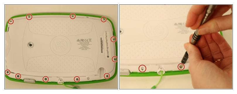
Remove the 11 Phillips screws (8.0 mm) located around the edge of the back cover with a Phillips screwdriver.
