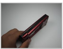
Using a plastic opening tool, separate the back cover from the phone.
