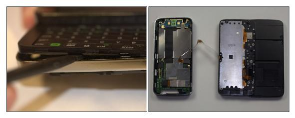
• Insert your spudger along the slit between the keyboard and the external casing. Pry open as shown.
