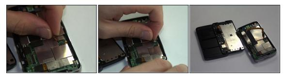
• Remove the keyboard ribbon from the motherboard. To do this, simply grasp the ribbon at its base and pry it up at an angle. The ribbon has a metal end that is easily removed from the motherboard.
