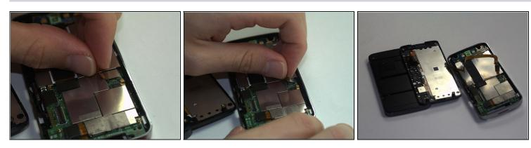
• Remove the keyboard ribbon from the motherboard. To do this, simply grasp the ribbon at its base and pry it up at an angle. The ribbon has a metal end that is easily removed from the motherboard.
