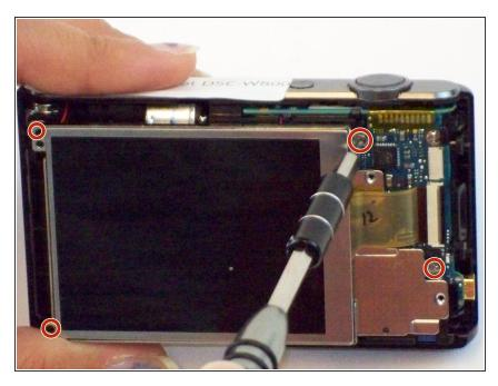
Remove the four 3.75 mm Phillips #000 screws from the LCD back panel.
