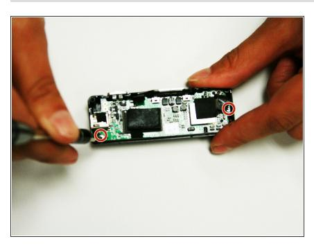
Using the PH000 drill bit from the iFixit toolkit, unscrew the two (2) screws to detach the motherboard from the device.
