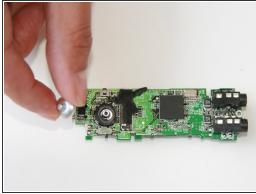
• The silver plastic cover to the joystick will be on the front side of the device. Pull the cover off with your hand.
