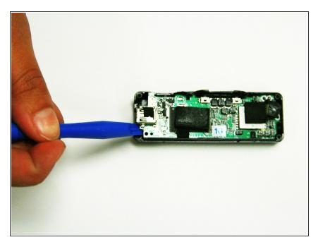
Wedge the plastic opening tool between the device case and the motherboard. Push down on the exposed end of the device, and the motherboard should pop up.
