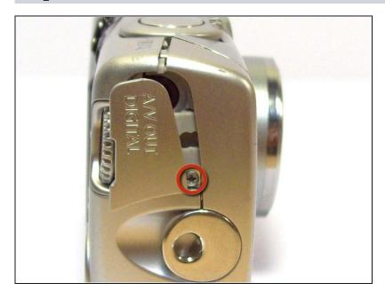
Use a Phillips #00 screwdriver to remove the screw on the left of the camera under the A/V out Digital label.
