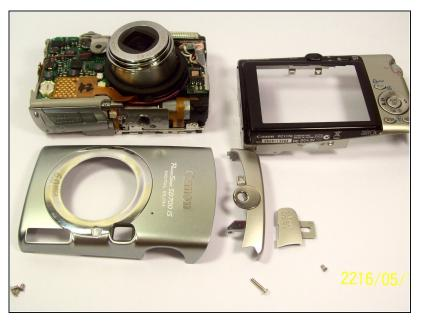
Remove the front, back, and side casings from the camera and set to the side.
