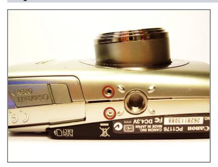
Remove the two, small screws on the bottom of the camera using a Phillip's #00 screwdriver.
