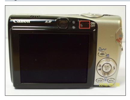
Turn off the camera by pressing the power button above the LCD screen.
