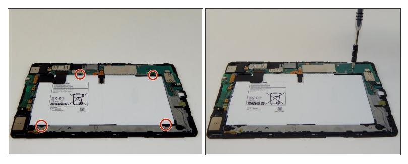
• Remove the four black 3 mm Phillips #1 screws that hold the battery in place.
