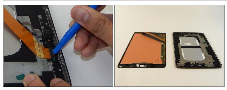
• With the plastic opening tool gently lift to disconnect the gold ribbon cable that attaches the screen to the base tablet.
