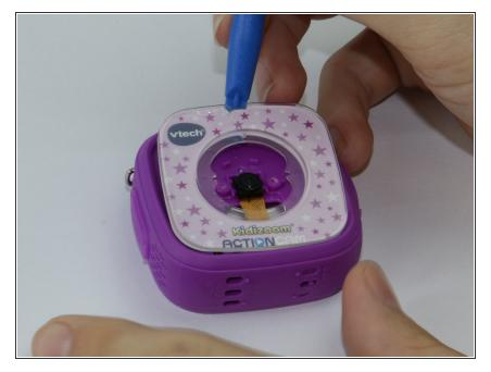
Pry off the transparent plating and paper design using a plastic opening tool.
