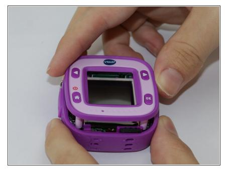
• Turn the camera around and gently remove the plating that surrounds the LCD screen by grasping it with your fingers and pulling away from the device.
