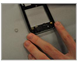
Use the spudger to pry out the grey rubber rectangular component from the main case.
