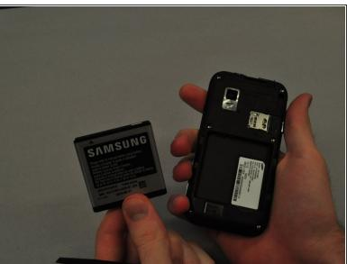
• Insert the spudger into the space between the battery and the phone and pry the battery out as you slide it along the underside the battery.
