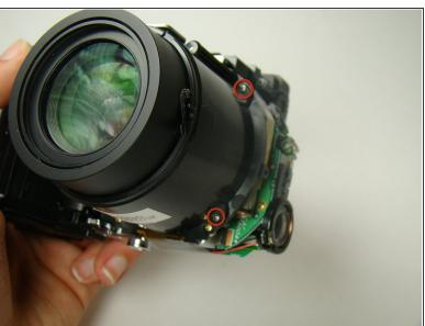
Remove the four black screws at the corners of the lens housing.
