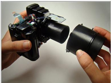
Remove the lens case and the lens.
