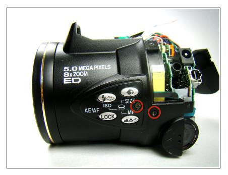
Remove the two screws on the left side of the camera.
