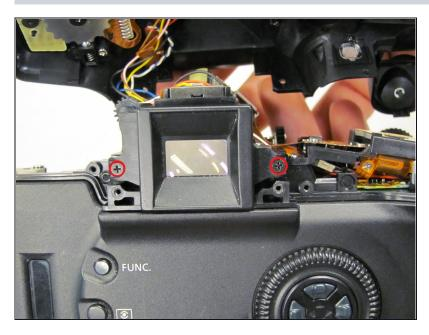
Remove the two 9.5 mm black screws that attach the inner eyepiece to the camera's body and remove the eyepiece.
