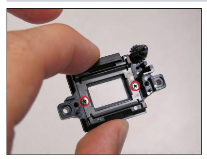
Remove the two 3.6 mm black screws from the outer piece.
