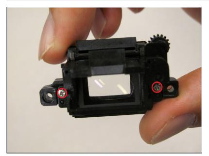
Remove the two 4.3 mm silver screws on each side of the inner eyepiece.
