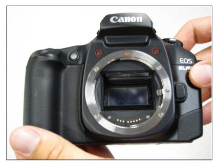
Remove the two 4.8 mm black screws above the lens on the front of the camera.
