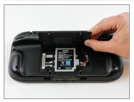
• Lift and remove the battery plate.
