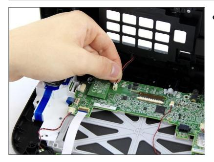
• Unplug outer case rumble motor connector from the motherboard with your fingers.
