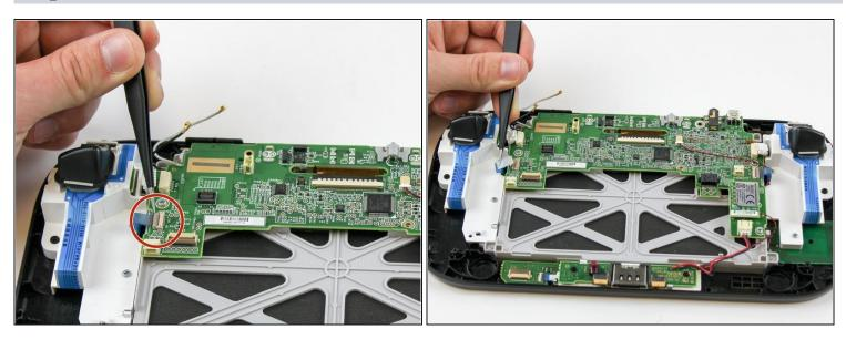
• Remove the blue connector using tweezers.
