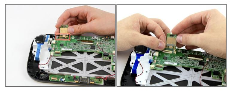
• Disconnect the black and white wires off of the back of the WiFi module.
