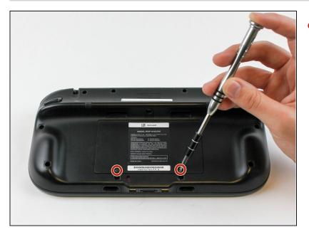
Place Gamepad face down and remove the two 4.7 mm screws with a Phillips size #00 screwdriver.
