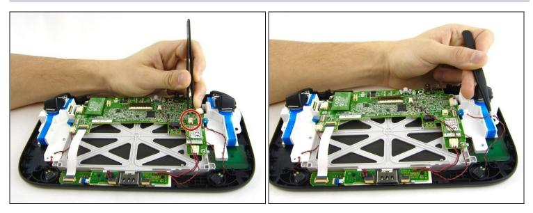
• Remove the right speaker cable that's connected to the motherboard with the <u>tweezers</u>.
