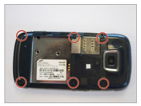
Remove the six 3.5 mm screws using a Phillips #000 screwdriver.
