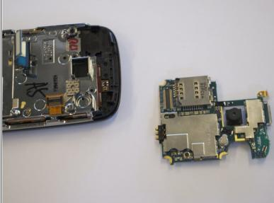
The circuit board will still be held on by a blue and black ribbon. Remove the entire circuit board by gently tugging the ribbon upwards.
