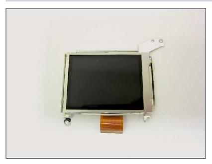
• The LCD screen can now be be removed to be fixed/replaced.
