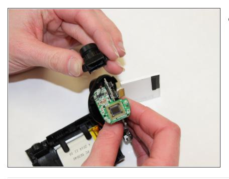
The lens should easily remove from the circuit board.
