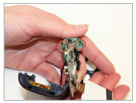
Behind the lens, use the metal screwdriver to unscrew the two screws holding the lens in place on the circuit board.
