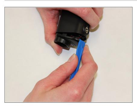
Use the plastic opening tool to pry off the front panel of the device.
