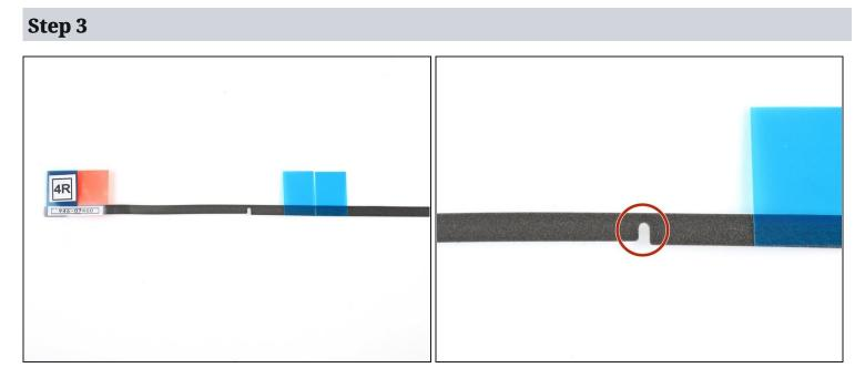
i Your adhesive strips should have a microphone notch pre-cut in the strip labeled 4R.
