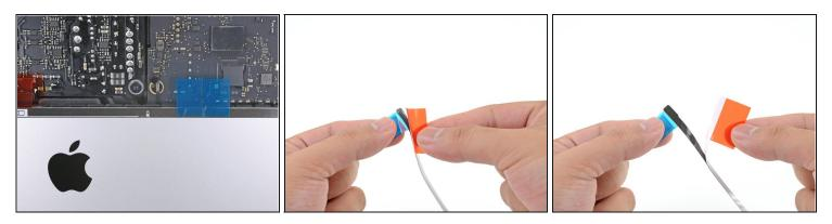
The next few steps will show you how to install the bottom right adhesive strip (strip 4R), which includes a notch that must be aligned with the microphone.
