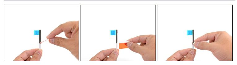
Fold the loose white backing to a right angle and pinch the crease with your fingers.
