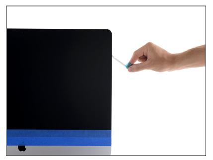
• Repeat the previous steps to remove the protective films from all the remaining adhesive strips.
