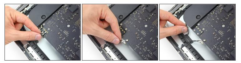
• Gently push the antenna cables aside to clear access to the AirPort/Bluetooth card.
