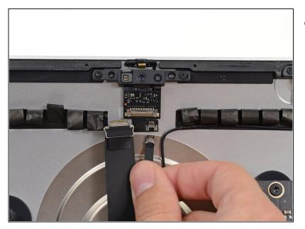
• Disconnect the microphone connector from its socket on the camera board.
