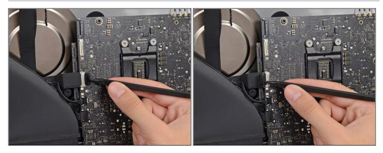
• Use the tip of a spudger to flip up the metal retaining bracket securing the camera cable connector to the logic board.
