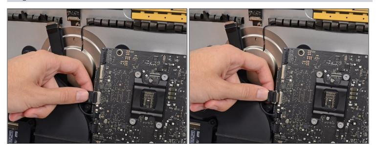
• Pull the camera cable straight away from its connector on the logic board.
