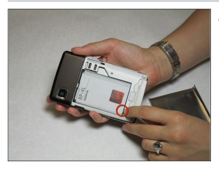
Locate the bottom-left corner of the phone where there is a spot to remove the battery.
