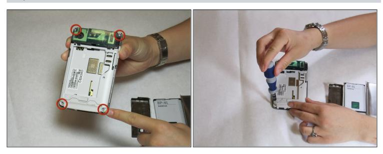
• Remove the four screws that secure the front cover to the rest of the phone using a T7 screwdriver.
