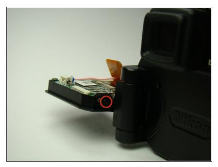
Remove the Phillips screw on the top right side of the screen.
