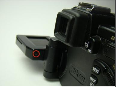
• Remove two Phillips screws (3.4 mm) located on the right side of the screens.
