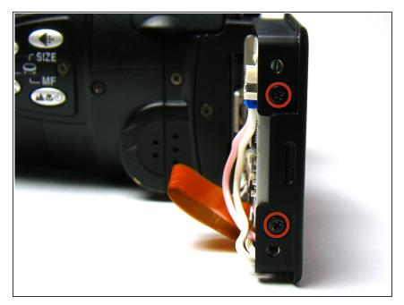
Remove the two Phillips screws on the left side of the screen.
