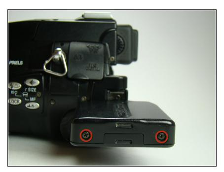
Remove two Phillips screws (3.4 mm) located on the left side of the screen.
