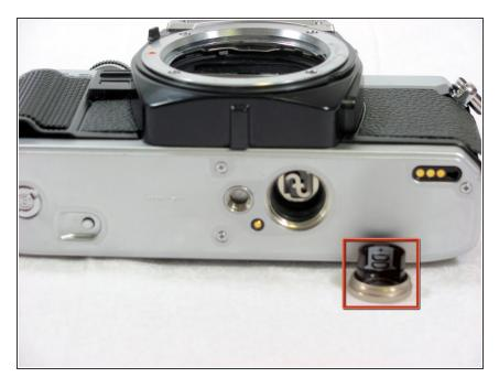
Remove the batteries, making sure to note their proper alignment.
