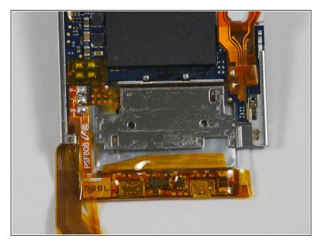
Unfortunately, the battery is soldered to the logic board.
