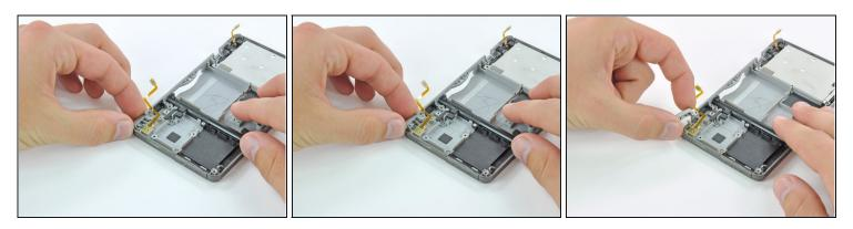
Press lightly on the back of the button until it becomes unattached. Be careful not to lose the small spring and pin behind the plastic button.
