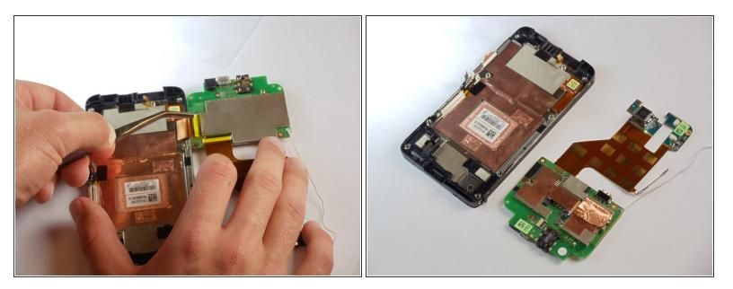
• With the back of the main board exposed, flip up the little brown lever at the end of the connector and unplug the final cable that connects it to the main board.
