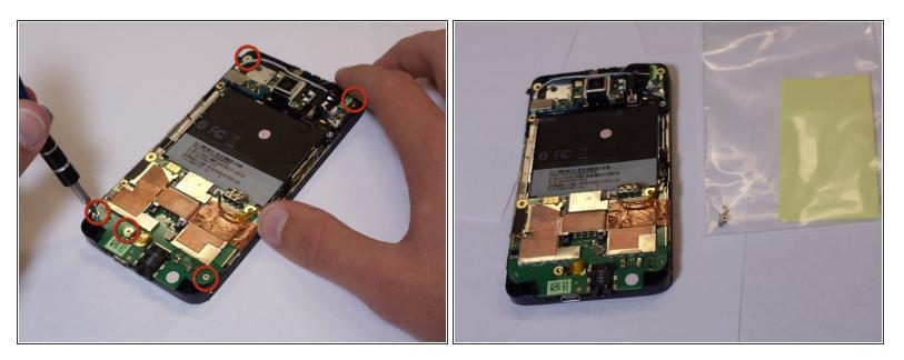
• Remove five T5 Torx screws from the motherboard.
