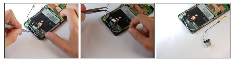
• Pull the camera flash and cover off of the board.
