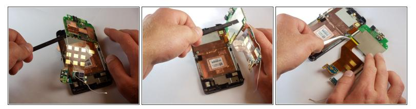
A There is a connecter cable under the main board, so do not pull it all the way off right away.
