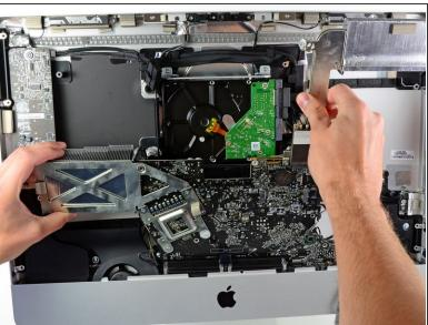
Slightly pull the logic board away from the back of the outer case, then lift it upward to clear the lower front face of the outer case.
