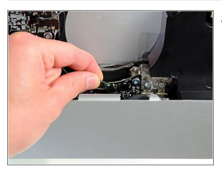
Pull the SD board cable out of its socket on the logic board.
