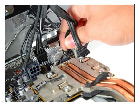
Pull the hard drive power cable connector out of its socket on the logic board.
