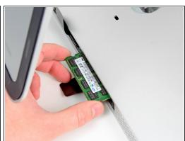
Repeat the process in the previous steps to remove the RAM module(s) from the other side of the RAM bay.
